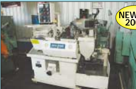
(3) Warren Model WT-1500 "1015" High Speed Flat Die Thread Rollers
