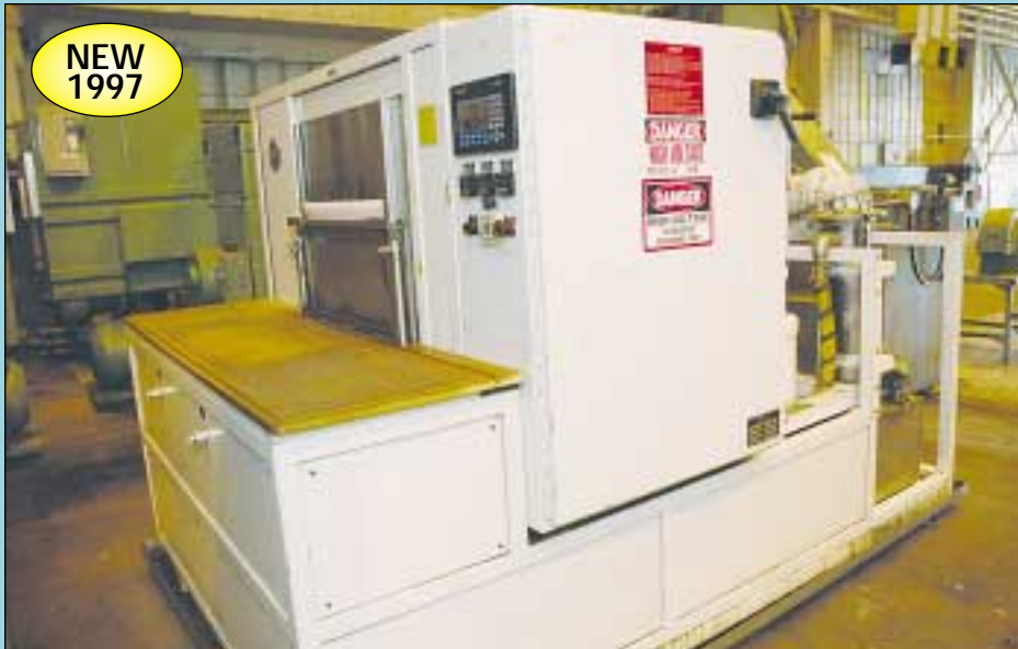
Better Engineering Model Cyclo-Jet III Basket Type Parts Washer
