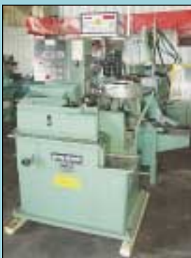
Warren Model WT-500 "00" High Speed Flat Die Thread Roller
