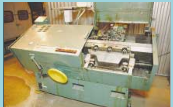
Hartford Model 10-400 High Speed Flat Die Thread Roller
