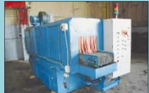
12" Wide X 96" Nobles Stainless Steel Two-Stage Continuous Mesh Belt Parts Washer
