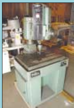
DoAll Model DTR23 Geared Type Radial Arm Drill
