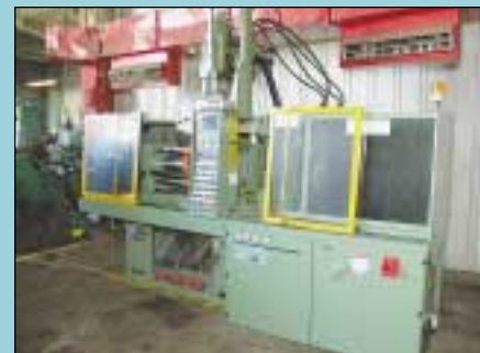
80 Ton Engel Model ES80/30 Horizontal/Vertical Hydraulic Injection Molding Machine
