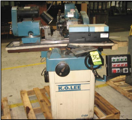
K.O. LEE C13A CYLINDRICAL GRINDER, S/N 28775
