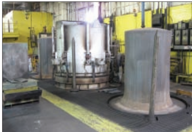
LEE WILSON BELL ANNEALING FURNACE CELL
