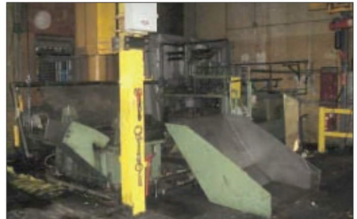
SCRAP BALER CHARGING BOX 44" (1117mm) X 96" (2438mm) x 22" (558mm) DEEP
