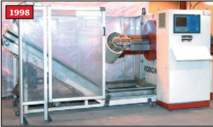
LATOUR ROBOMAC 310 3 plane, 5 axis CNC wire forming machine
