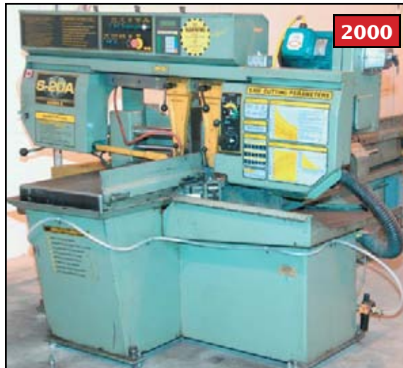
HYD-MECH S20A fully automatic horizontal bandsaw
