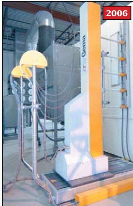
ITW GEMA ZA04-18 reciprocators with 5 guns
