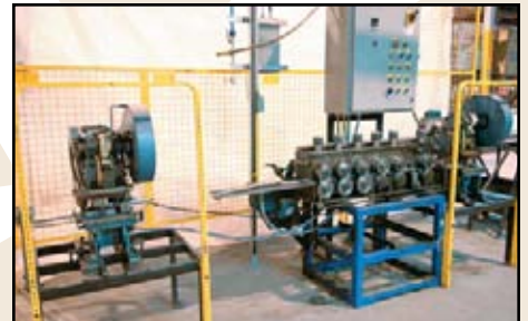
RGA 6 station channel forming line
